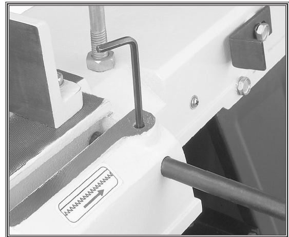
Figure 17. Installing the work stop shaft.
